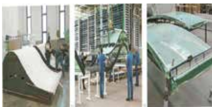
Figure 3 Process of cold bending of glass - on the substructure, in the factory (Molter & Wolf, 2011).
